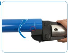
Rotate the jaw to apply the next lug. The circle showsthe alignment mark made by the jaw from the
