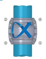
For effective assembly, tighten the screws in an "X" pattern. To disassemble, perform the same operation in reverse order.
