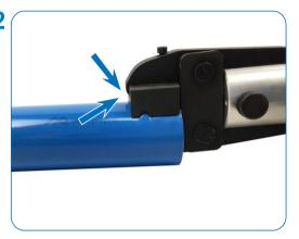
Press the trigger on the lugging tool to run the lugging cycle. A "snap" sound is made when the applied lug is completed.crimp the pipe until a "snap" sound is heard.
