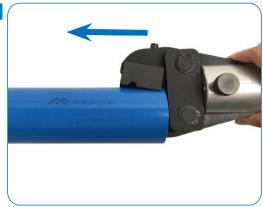
Open the jaw and insert the pipe completely.
